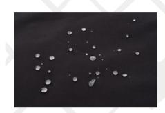
335GSM,3 layer bonded fabric, 75D 95%polyester 5%spandex + membrane film + 96D/144F Micro fleece on back. Waterproof and Breathable
